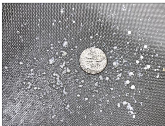
Figure 3. Fox Valley 32/40 residue remaining on 500 \mu m sieve after water spray to break surface tension.
