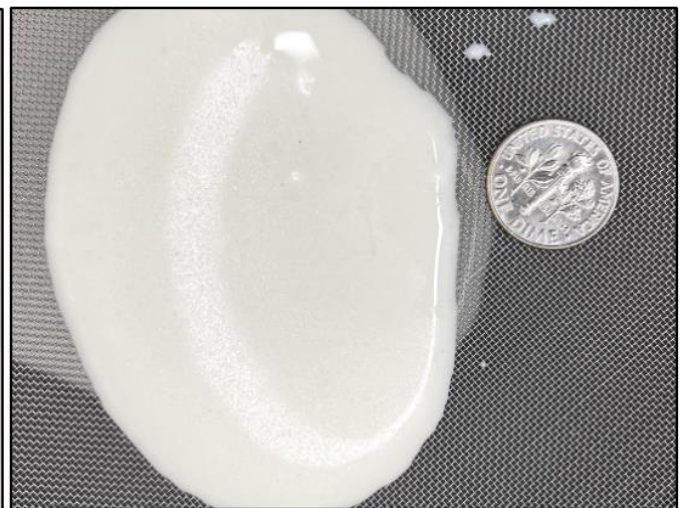
Figure 2. Fox Valley 32/40 formula poured onto 500 \mu m sieve. Suspended on mesh by surface tension.
